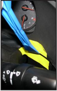
d. Use panel safe tool to pull out knee bolster. (Fig. 11-3)
