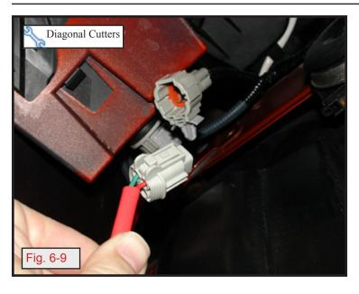
j. Reassemble turn signal connector and reattach to vehicle. (Fig. 6-9)
