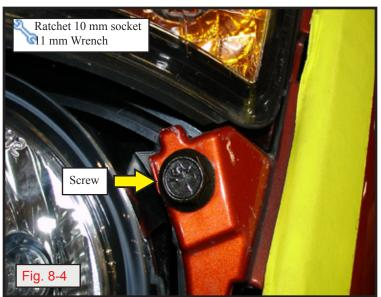
d. Insert screw from front and nylock from the back. Use 10 mm socket on the front and the 11 mm wrench on the back. (Fig. 8-4)
