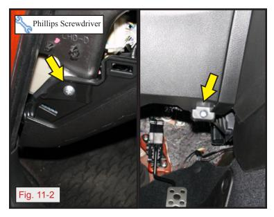
c. Remove one (1) screw located under side panel, and one (1) screw located at the right bottom of the knee bolster panel as indicated by arrows. (Fig. 11-2)
