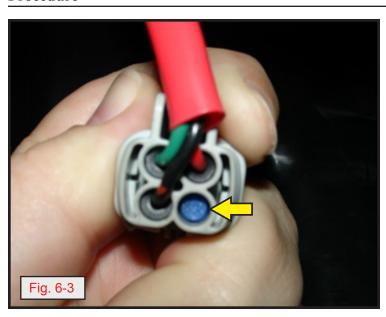
d. Locate blue plug on turn signal side connector. (Fig. 6-3)
