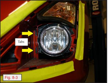
Insert light assembly from inside of bumper then shift inboard to seat inboard retaining tabs into slots indicated by arrows on bumper cover. (Fig. 8-3)
