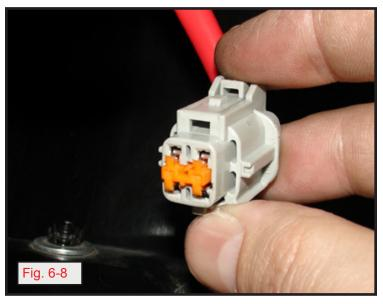
i. Replace orange retainer and press into place. (Fig. 6-8)
