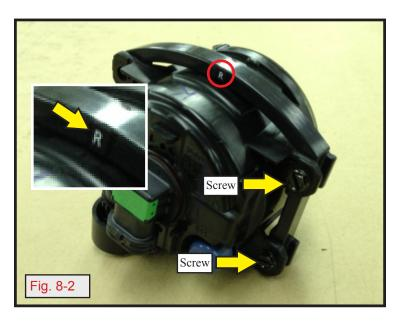
b. Assemblies will now be handed and are marked left and right on top part of adapter bracket. (Fig. 8-2)
