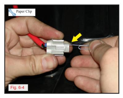
e. Insert a paper clip in front of connector to remove blue plug, discard plug. (Fig. 6-4)
