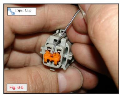
f. Remove orange locking tab from front of connector using a paper clip. (Fig. 6-5)
