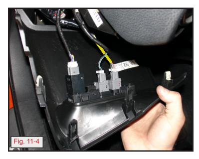
e. Disconnect all connectors and remove from vehicle. (Fig. 11-4)
