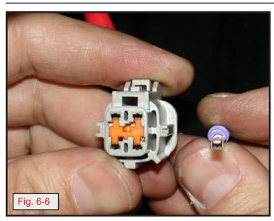
g. Insert terminal with purple seal from fog light harness into open cavity of turn signal connector. (Fig. 6-6)
