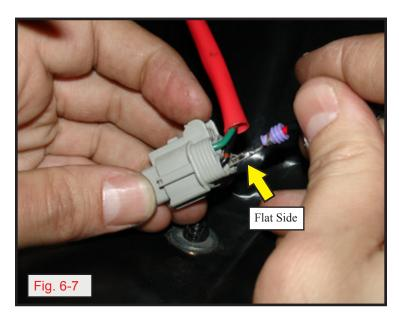
h. Flat side of terminal goes toward outside of connector as indicated by arrow. Make sure to align and properly snap in. (Fig. 6-7)
